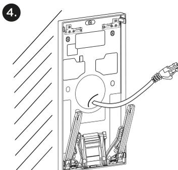
Drill chassis anchoring holes on a proper place. Use the chassis itself as a template to maintain the horizontal level and carry the cabling at the bottom edge of the cable hole. The recommended length of the accessible cables is 35 cm (1).
