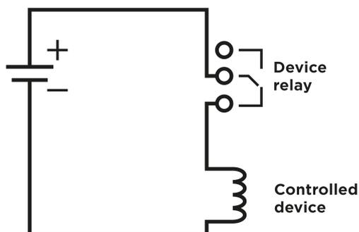
Wiring diagram for breaking of the electric circuit of the device to be controlled
