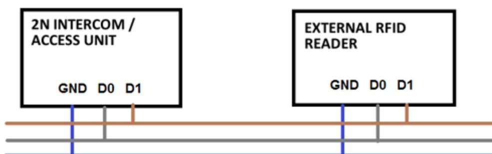
Recommended reader - bus driver wiring diagram
