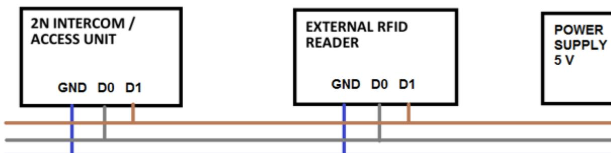
Recommended reader wiring diagram with OC output
