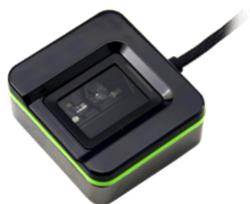
2N<sup>®</sup> IP intercom- external fingerprint reader (USB interface)
